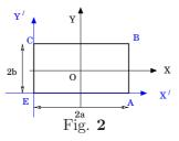
$$I_{xx} = \int_{-a}^{a} dx \int_{-b}^{b} dy \sigma y^{2} = \int_{-a}^{a} dx \sigma \frac{2b^{3}}{3} = \sigma \frac{2b^{3}}{3} \int_{-a}^{a} dx$$
